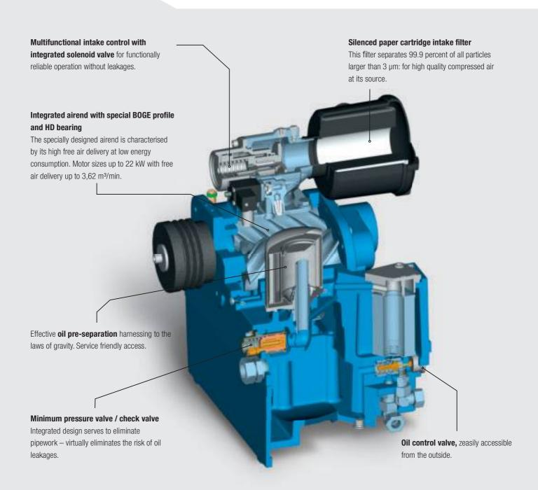
The state-of-the-art compressor: Extremely quiet, compact & efficient — the "large" BOGE C series has set industry standard in specific power and sound pressure values. The BOGE compact module enables short distances and less pipelines - for a highly efficient and reliable compressor solution. Depending on your requirements, the C series up to 22 kW can be equipped with refrigerant dryer, frequency control or heat recovery: This is the way compressors are made today!
